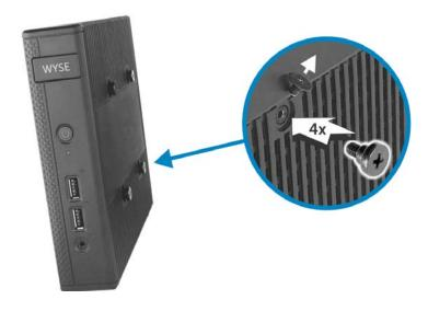
**2.** Attaching E Bracket to the Monitor - Remove the four (4) VESA screws from the back of the monitor and set them aside. Position the E bracket on the back of the monitor and attach it using the same VESA screws (do not over-tighten).
