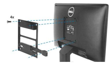
**3.** Attaching the Client - Place the monitor in the upright standing position. Then, slightly tip the client to align and insert the four protruding shoulder screws into the four cutout areas of the E bracket. The security latch will move automatically when the shoulder screws are inserted.
