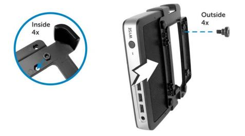
2. Attaching the E Bracket to the Monitor - Remove the four (4) VESA screws from the back of the monitor and set them aside. Position the E bracket on the back of the monitor and attach it using the same VESA screws (do not over-tighten).
