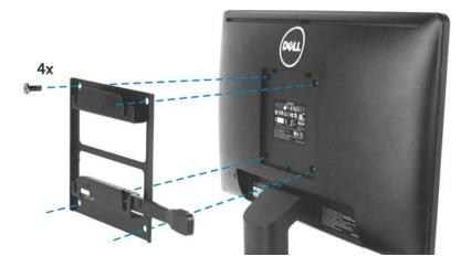
**3.** Attaching the Client - Place the monitor in the upright standing position. Then, slightly tip the client to align and insert the protruding shoulder screws into the four cutout areas of the bracket. The security latch will move automatically when the shoulder screws are inserted.
